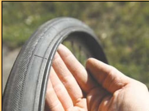
Figure 3: Run fingers inside to find debris.
