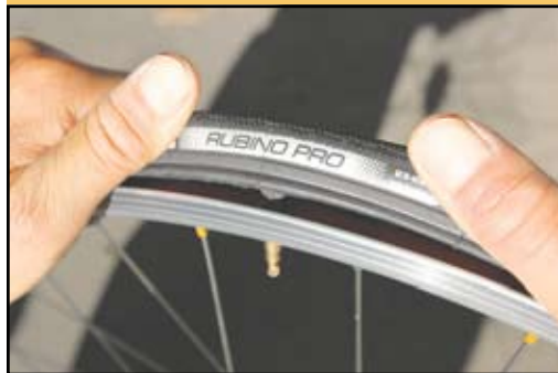
Figure 1. Roll tire back to expose bead.
