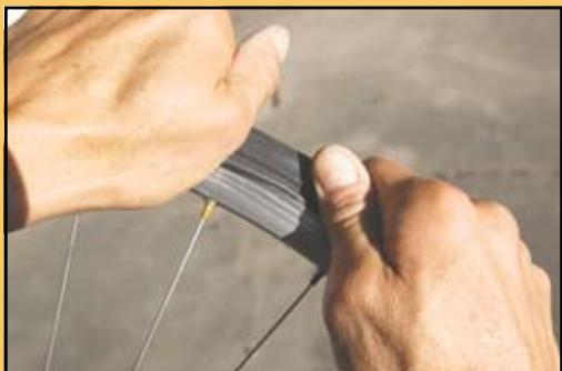
Figure 4: Roll bead over with palm and thumb.
