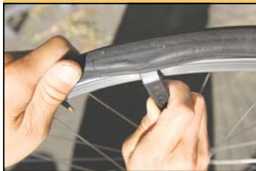
Figure 2. Insert tire lever and pry up.
