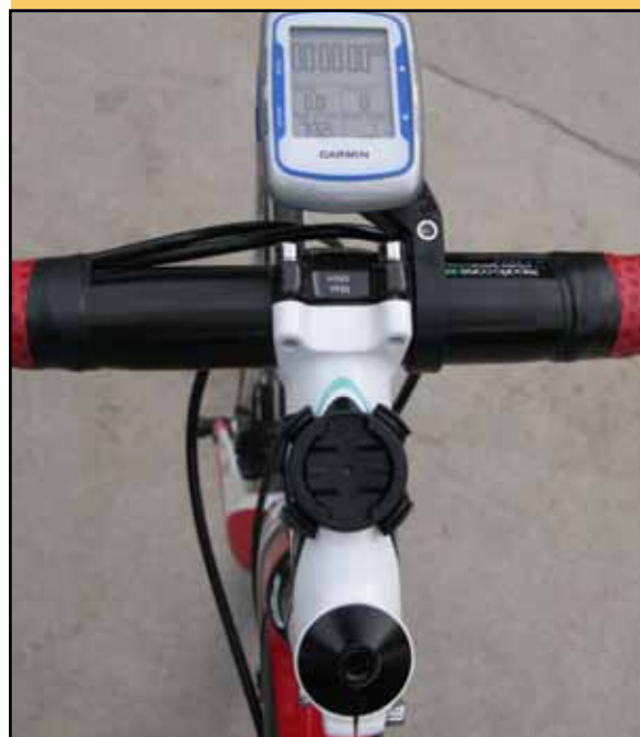
Above: The Bar Fly (front) is a great alternative for mounting a Garmin Computer. The stock Garmin mount is shown for comparison on the stem.
