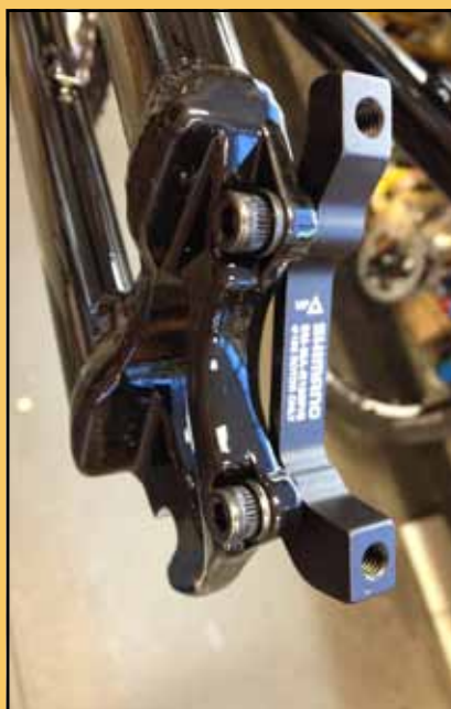
Top: Brake line inside frame. Middle: Brake rotors 160mm (L) 180mm (R). Below: Installing the olive and barb. Bottom left: International standard (IS) mount. Bottom right: Trim cable ties.
