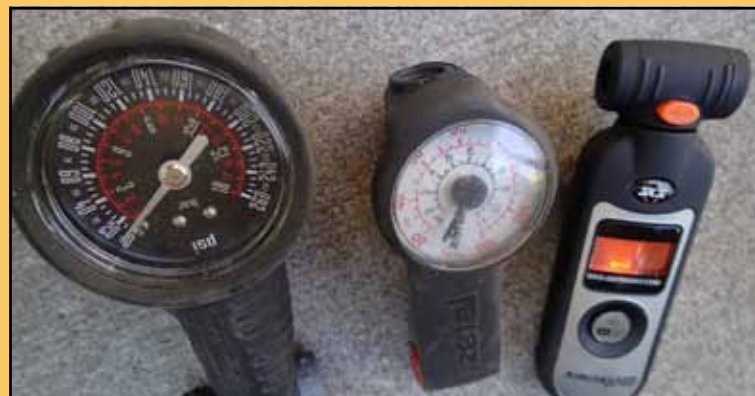
Three tire pressure gauges. I pumped up a MTB tire with my favorite pump. The tire pump read 30 psi. One gauge read 27.5, the second 36 and the third 40. Which is accurate? It really doesn't matter. Use the same gauge every time and learn what psi works for you.
