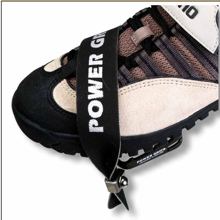
A Power Grip with the foot in the pedal. Photo courtesy MRP
