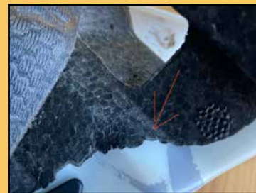
A small crack in Tom’s helmet from a crash, not visible from the outside. Photo by Tom Jow
