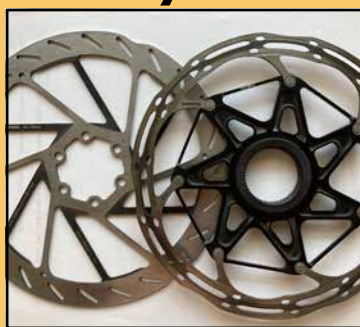
Photo 3. Two types of rotor mounts. Centerlock rotor (right) slides onto splines on the hub. Photo by Tom Jow
