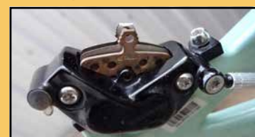
Photo 6. Gently pull up to remove the brake pads. The type of friction material is on the backing plate. Photo by Tom Jow
