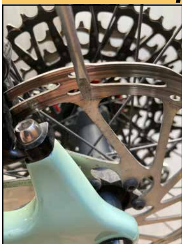
Photo 1. A small screwdriver is helpful to test the rotor surface. Photo by Tom Jow
