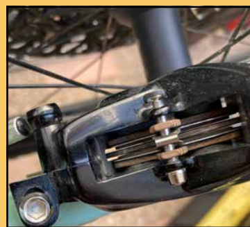
Photo 4. Look into the caliper to quickly check the brake pad thickness. Photo by Tom Jow
