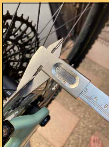
Photo 2. Use a metric caliper to find the exact thickness of the rotor. The minimum thickness will be printed on the side of the rotor. Photo by Tom Jow
