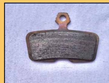
Photo 5. A well-worn brake pad. Notice deep grooves, pits, and chips on the brake pad surface. Photo by Tom Jow
