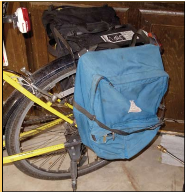
Above: Commuting bike setup with rear flashing light, kickstand, panniers, and rack.
