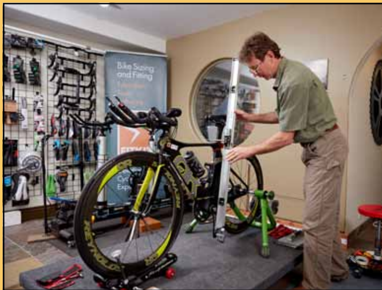
John Higgins measures saddle height at the Bike Fitr studio. Photo by Derek Israelsen Photography
