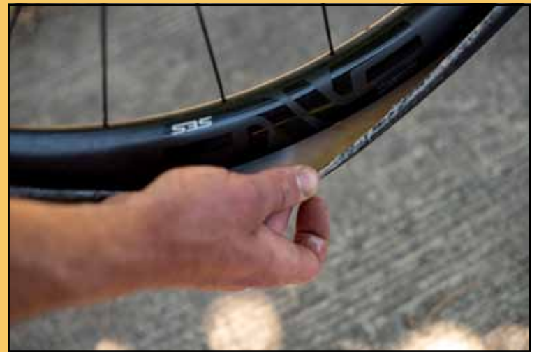
Road tubeless tires need sealant, but are easy to take on and off. Photo by Ian Matteson - ENVE Composites
