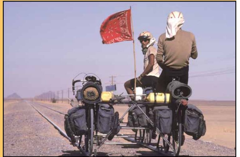
In northern Sudan on the Too Tired Bike Tour, with no road to Egypt, Tim Young and his co-travelers modified their bikes to ride on the old British narrow gauge rail line. It took 10 days to build the parts, and a couple weeks to ride across the Nubian Desert. Photo courtesy Tim Young
