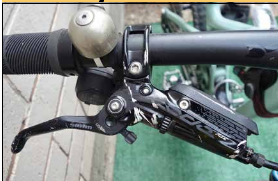
A well used mountain bike brake lever. The large bulge on the right is the master cylinder. The knurled dial in the lever body adjusts the brake pad contact point. The knob on the brake lever adjusts the static or resting position of the lever. Photo by Tom Jow
