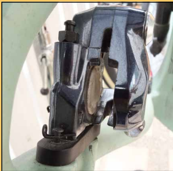
Inside view of a lightweight road disc caliper. One of the two pistons is exposed without brake pad. The external bleed port protrudes from the top of the caliper. Photo by Tom Jow
