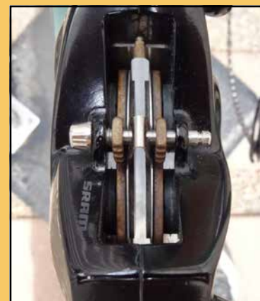
Inside view of a heavy duty mountain bike brake. Notice the two pistons extended from the caliper body on each side behind the brake pads. Photo by Tom Jow
