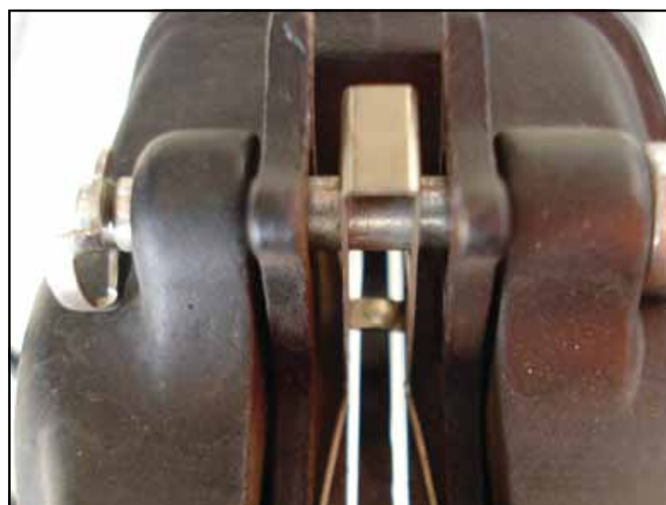
There should be a lot of room between the brake pads and the disc rotor.
