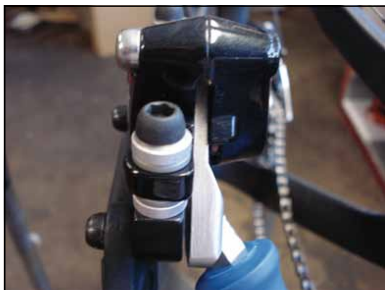
Use a brake piston tool (Park PP-1) to reset and lube the brake pistons.
