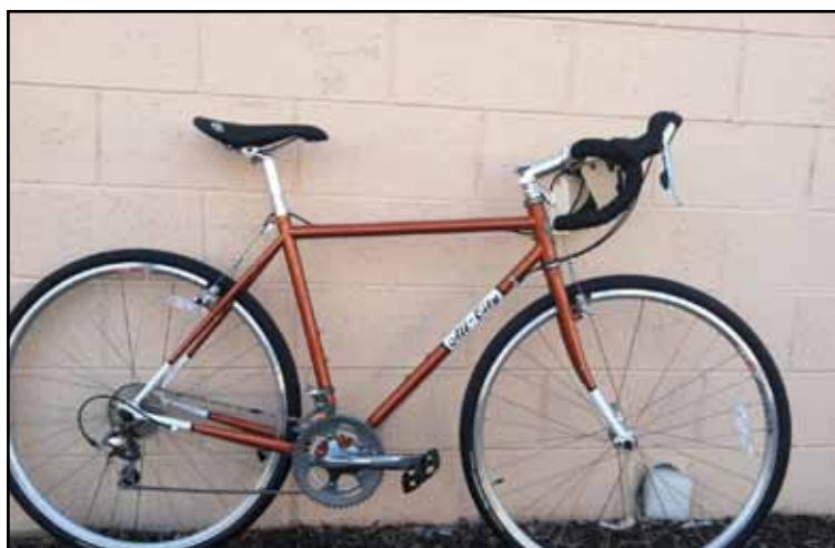
Above: The All City SpaceHorse is a sport-touring bike that has mounts for racks, fenders, and waterbottles and room for large tires and makes a great longer distance commuter.
