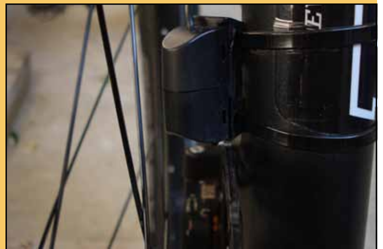
The accelerometer and sensor and sensor work to adjust the suspension in response to the terrain.
