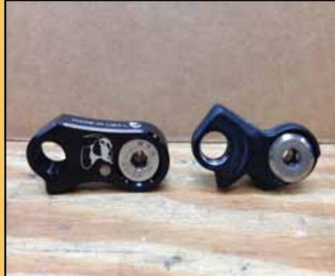
Top Left: Rear derailleur without the Goat Link (left). Rear derailleur with the Goat Link (right). Top Right: The Goat Link works to convert a rear derailleur into one that will work with a larger cog, and a single front chainring. Below Left: The c-clip must be removed in order to install the Goat Link.
