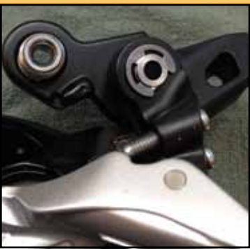
Top Left: Rear derailleur without the Goat Link (left). Rear derailleur with the Goat Link (right). Top Right: The Goat Link works to convert a rear derailleur into one that will work with a larger cog, and a single front chainring. Below Left: The c-clip must be removed in order to install the Goat Link.
