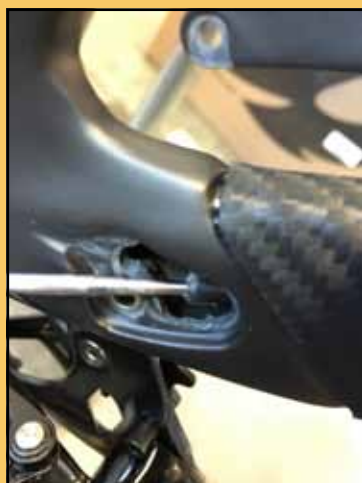
Guiding cable housing through a chainstay port. Photo by Tom Jow
