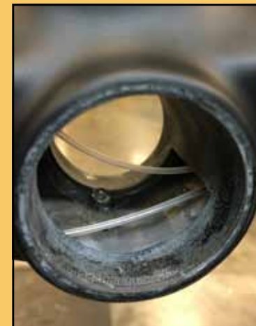
Cable liners shown in the bottom bracket shell. Photo by Tom Jow
