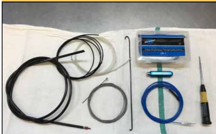
Various tools required to thread internal cables and brake lines. Photo by Tom Jow
