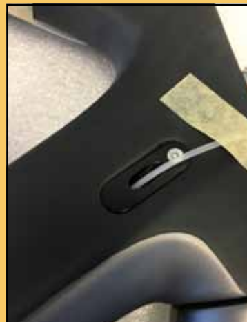
Plastic liner exiting cable stop port. Photo by Tom Jow
