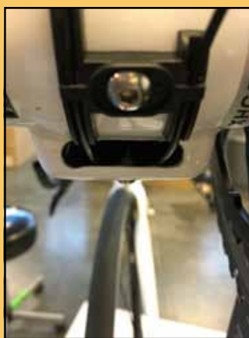
Cables of an interrupted cable routing exiting the downtube in front of a cable guide. Photo by Tom Jow
