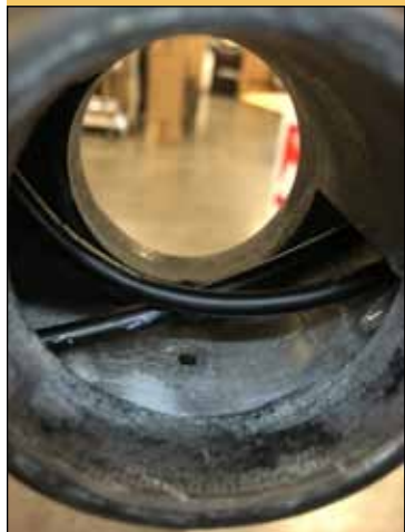
Open tube full cable housing style. The housing fits in between shell and bottom bracket. Photo by Tom Jow
