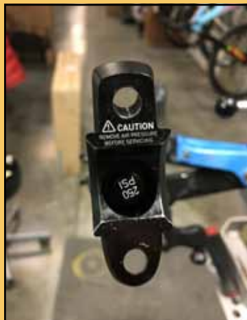
The air valve is located under the seat clamp. Photo by Tom Jow
