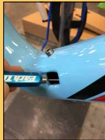
Using a magnet to pull a cable out of a downtube port. Photo by Tom Jow
