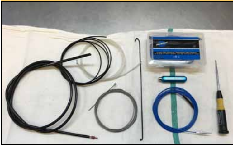
Various tools required to thread internal cables and brake lines. Photo by Tom Jow
