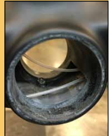
Cable liners shown in the bottom bracket shell. Photo by Tom Jow
