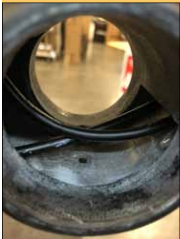
Open tube full cable housing style. The housing fits in between shell and bottom bracket. Photo by Tom Jow
