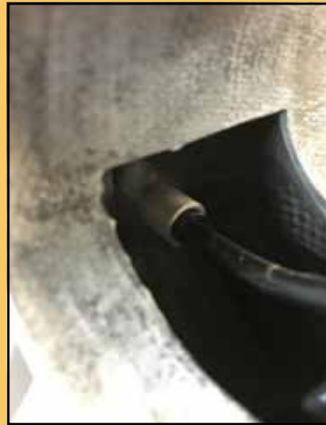
Example of a cable housing stop inside the bottom bracket shell. Impossible to insert with bottom bracket in place. Photo by Tom Jow
