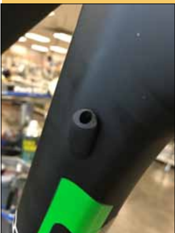
Rubber frame grommet keeps cable housing in place and seals frame opening. Open tube style. Photo by Tom Jow
