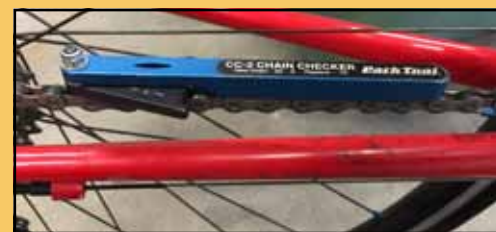
Checking chain 'stretch'. Photo by Eric Ramirez
