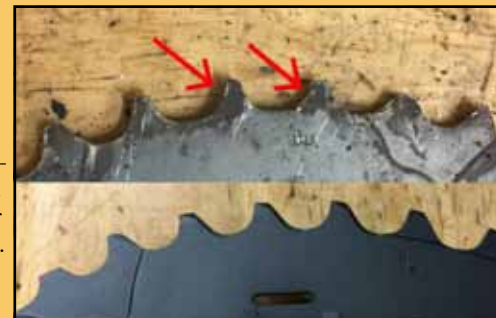
Used cassette teeth show mashed metal; an unusual lip can be felt moving across the tooth. Photo by Eric Ramirez
