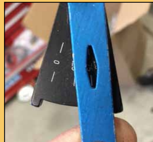
Usually when this tool displays 0.75 chain replacement is recommended. Photo by Eric Ramirez
