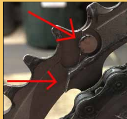
Ramps and pins shown here have signs of rounding and thus lose the ability to shift cleanly. Photo by Eric Ramirez
