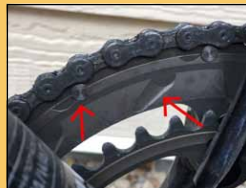
Identifying the shifting workhorses of chainrings (ramps are also found on cassettes). Photo by Eric Ramirez
