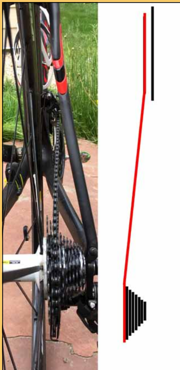
This exaggerated illustration shows how the chain flexes laterally in the climbing gear combo. Photo by Eric Ramirez
