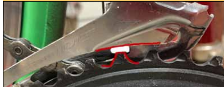
Vertical alignment: The gap between the bottom of the outer derailleur plate and the top of the teeth of the big chainring should be 1-3mm (gap indicated by white space). Photo by Eric Ramirez
