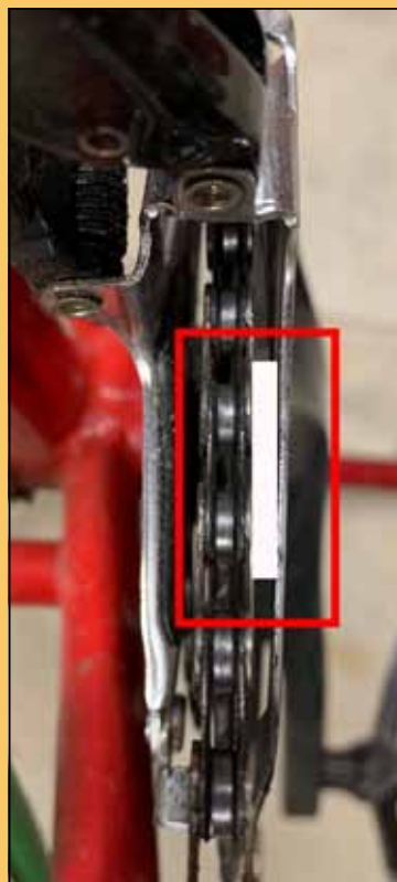
High Limit Gap: 2-3mm (white space) – Notice the chain sitting on the chainring is also parallel to the derailleur plates. Photo by Eric Ramirez
