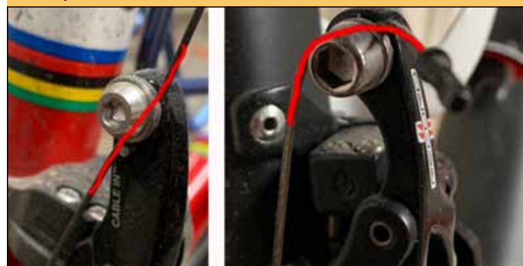
Cable Install: (left) Shimano Gen 2 Cable fixation; (right) Campagnolo cable fixation. Photo by Eric Ramirez
