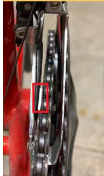
Low Limit Gap: The low limit gap (white space) between the inner face of the inside derailleur plate and chain should be roughly 2mm. Photo by Eric Ramirez
