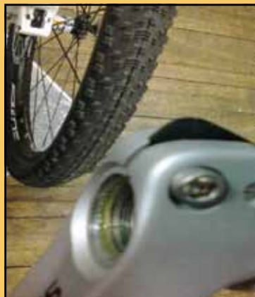
(Photo 1) Safety washer up, arm ready for removal.
