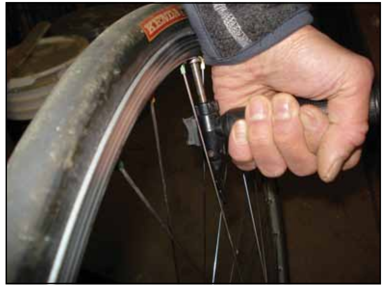
Keep pump perpendicular to the valve and brace against rim to prevent breaking the valve off.
