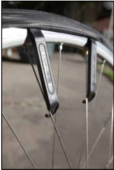
Use tire levers to pry the tire off the rim.
