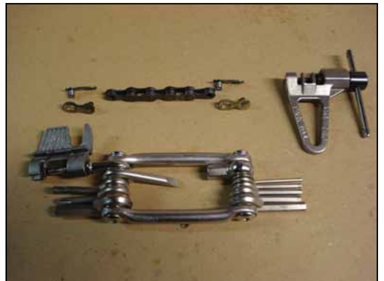
Multi-tool w/ integrated chain tool, chain tool and spare chain with repair links.
