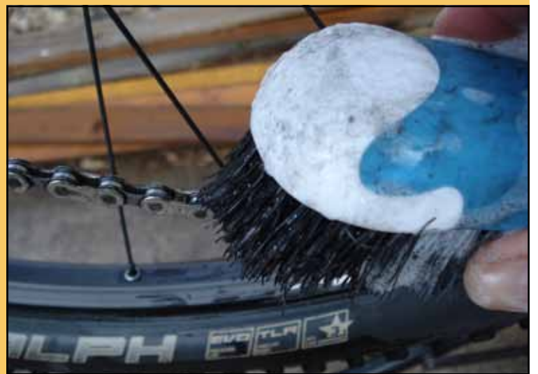
Top: Wash under the head tube. Second from top: Be sure to clean the cassette. Third from top: An old chain looks new after scrubbing the side plates. Bottom: Use your dirty brush on the chain rollers.
