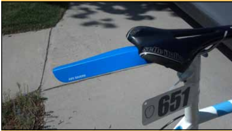
The Ass Saver is a simple clip-on rainguard that helps keep you dry. Photo: Jared Eborn
