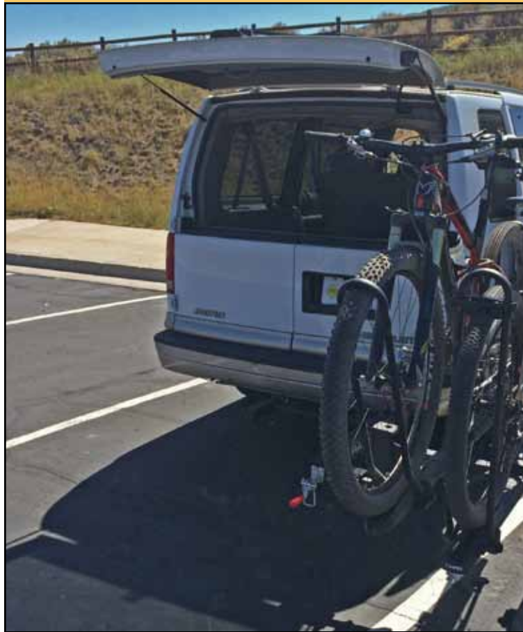
The RakAttach is a swing-arm that allows easy access to the tailgate when used with rear mount bike racks. Photo by Chris Magerl
