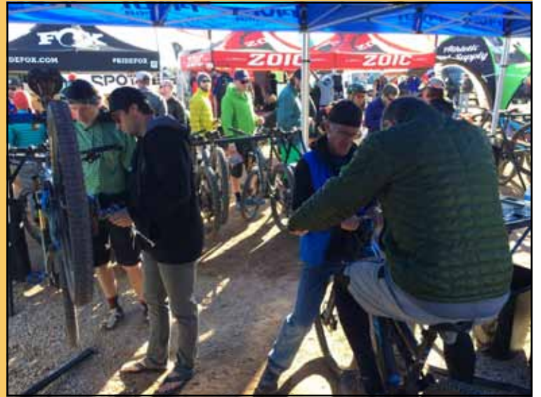
Pivot mechanic Brad Pastir, second from left, installs pedals on a demo bike about to be ridden by John Shuld of Chicago. On the right, Pivot's Tom Noaker steadies the bike to set front and rear sag for Romuald Mineyko of Montreal. You bring your pedals and the bike folks set up the bike to your weight, height and riding style. Photo by Chris Magerl
