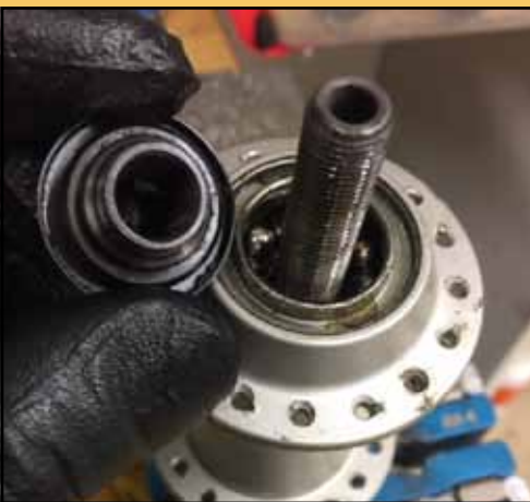
If your hub bearings are cup and cone, inspect the cones for pitting. Regrease and replace as needed. Photo by Eric Ramirez
