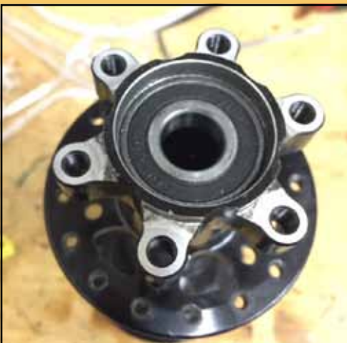
If your hubs have sealed bearings, inspect and replace as needed. Photo by Eric Ramirez
