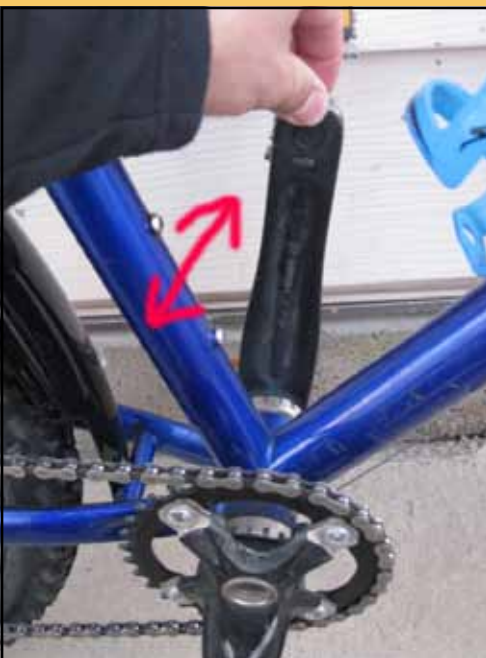
Check the bottom bracket bearings by feeling for play in the crankarms. Photo by Eric Ramirez
