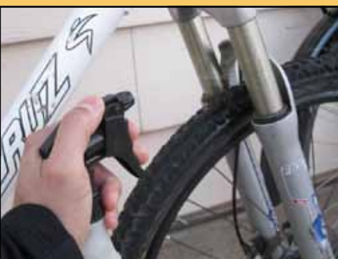
Spray off the stanchion tubes with isopropyl alcohol. Photo by Eric Ramirez
