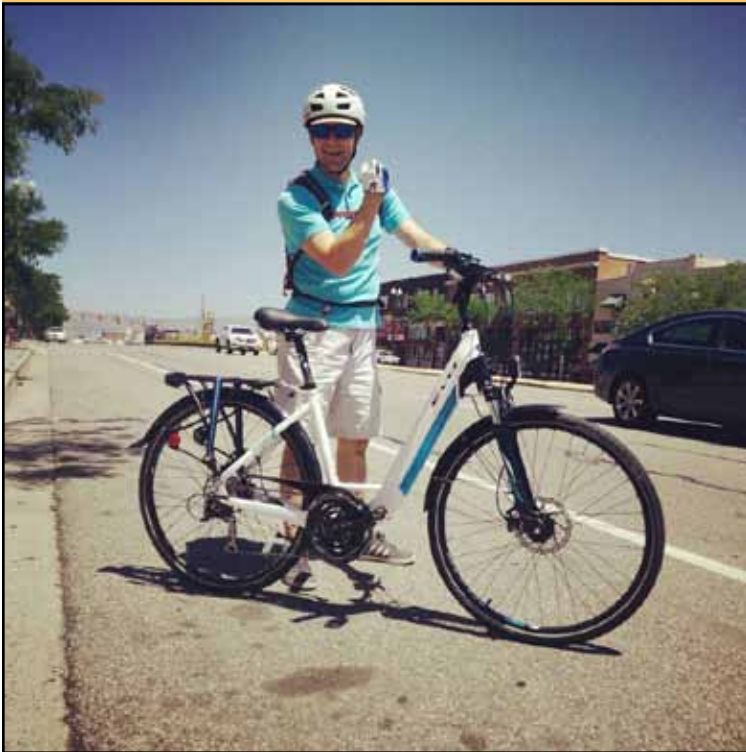
Mikey Geurts on an upright commuter e-bike with rear hub drive. Photo by Duane Schaffer
