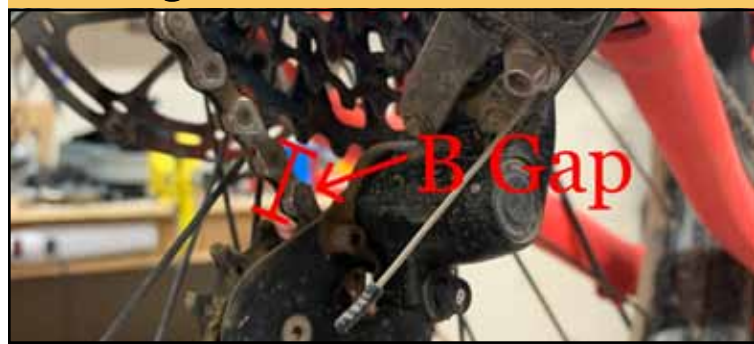
B-Gap is always measured when the drivetrain is in the absolute (easiest) climbing gear. In this case, the 1x11 drivetrain is oriented with the chain and derailleur in the 42 tooth position. The measurement is tooth to tooth, as seen here. Photo by Eric Ramirez
