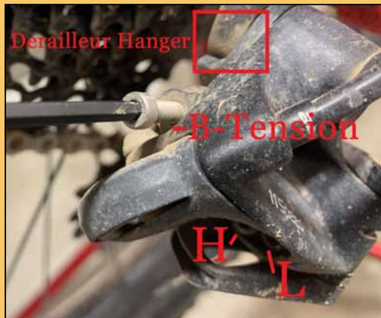
The B-Tension Screw almost always contacts the frame directly or indirectly. The part of the frame it contacts is called the derailleur hanger or derailleur tab. Photo by Eric Ramirez
