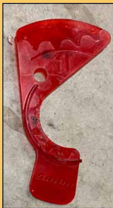
SRAM designed this handy tool for setting the B-Tension on their Eagle drivetrains (12 speed, single chainring, 10-50 tooth). Photo by Eric Ramirez
