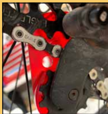
SRAM's tool in action - The lines clearly show where to hold the tool. The Silhouette matches the jockey pulley and 50 tooth cog. Photo by Eric Ramirez
