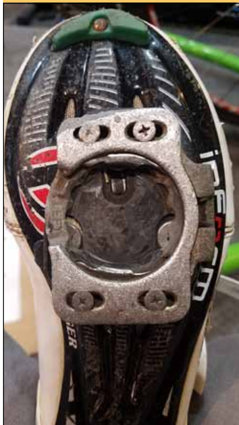
Worn bike cleats don't work very well, and sometimes keep you stuck to your pedals. Photo by John Higgins
